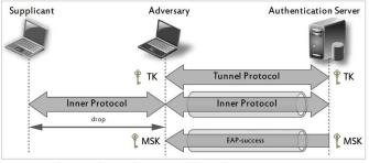
Fig12. MiTM in Tunnel based EAPs [11]
