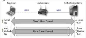
Fig 3. Tunnel based EAP type overview
