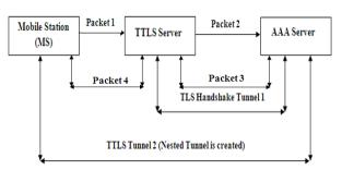
Fig14. EAP-TTLS Module Design
