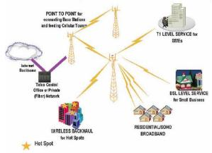
Fig 2. WiMAX Architecture and Applications
