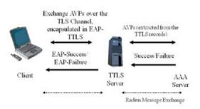
Fig7. EAP-TTLS Phase II
