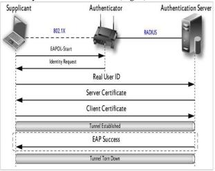
Fig 4. EAP-TLS Authentication
