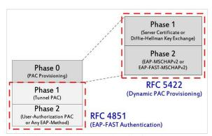
Fig9. EAP-FAST Authentication Phases
